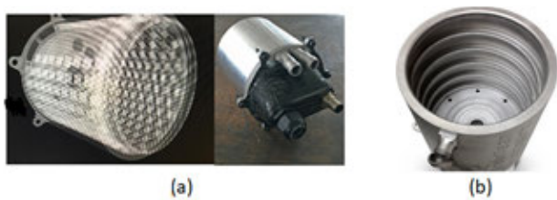
FIGURE 17. Two concept designs of liquid cooling jacket integrated into the housing and built by AM technology for racing car motor (a) TU fast racing team prototype [58], and (b) Greenteam Stuttgart prototype [59], and [60].
