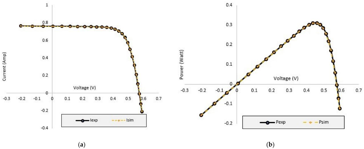
**Figure 6.** Characteristic curves for R.T.C. France SDM based on parameters extracted from TFWO: (a) Current–voltage (I–V) ch/s and (b) power–voltage (P–V) ch/s.
