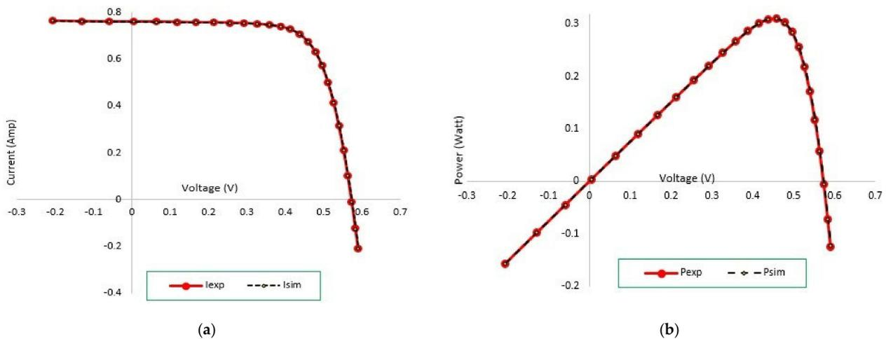
Figure 14. Characteristic curves for R.T.C. France TDM based on TFWO: (a) I–V ch/s and (b) P–V ch/s.
