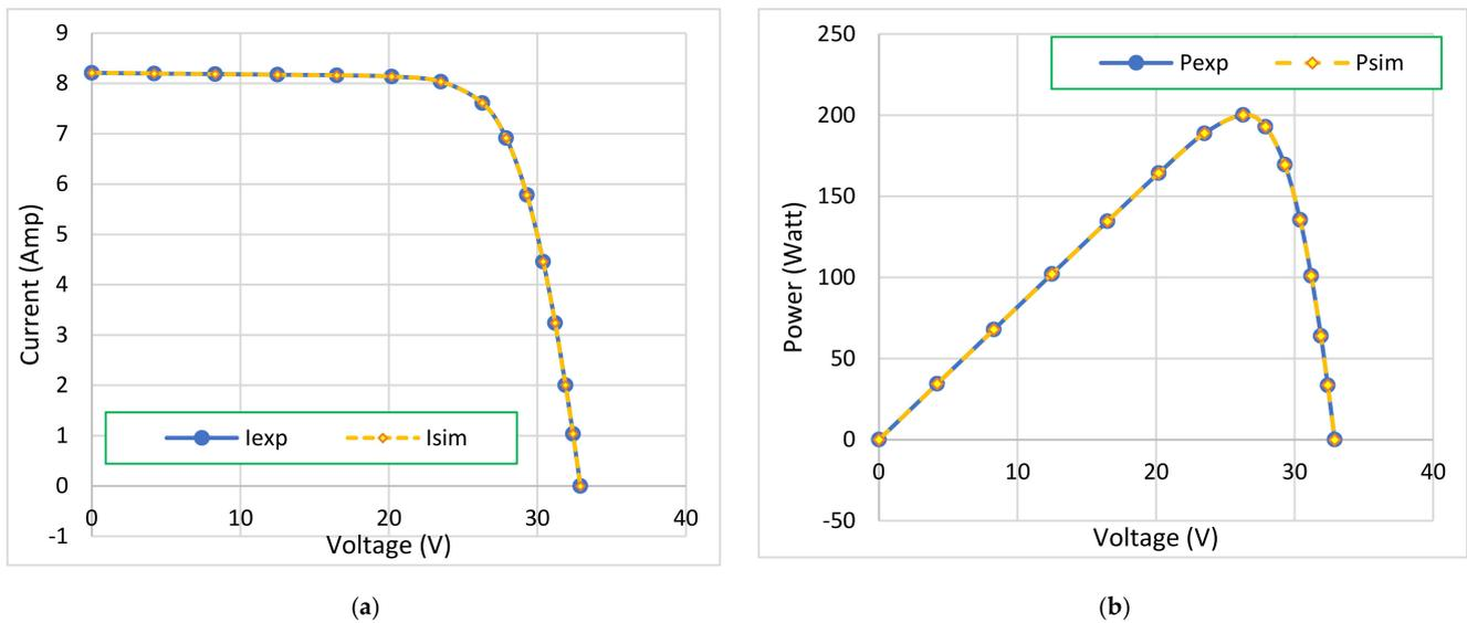
Figure 18. Characteristic curves for KC200GT SDM based on TFWO: (a) I–V ch/s and (b) P–V ch/s.
