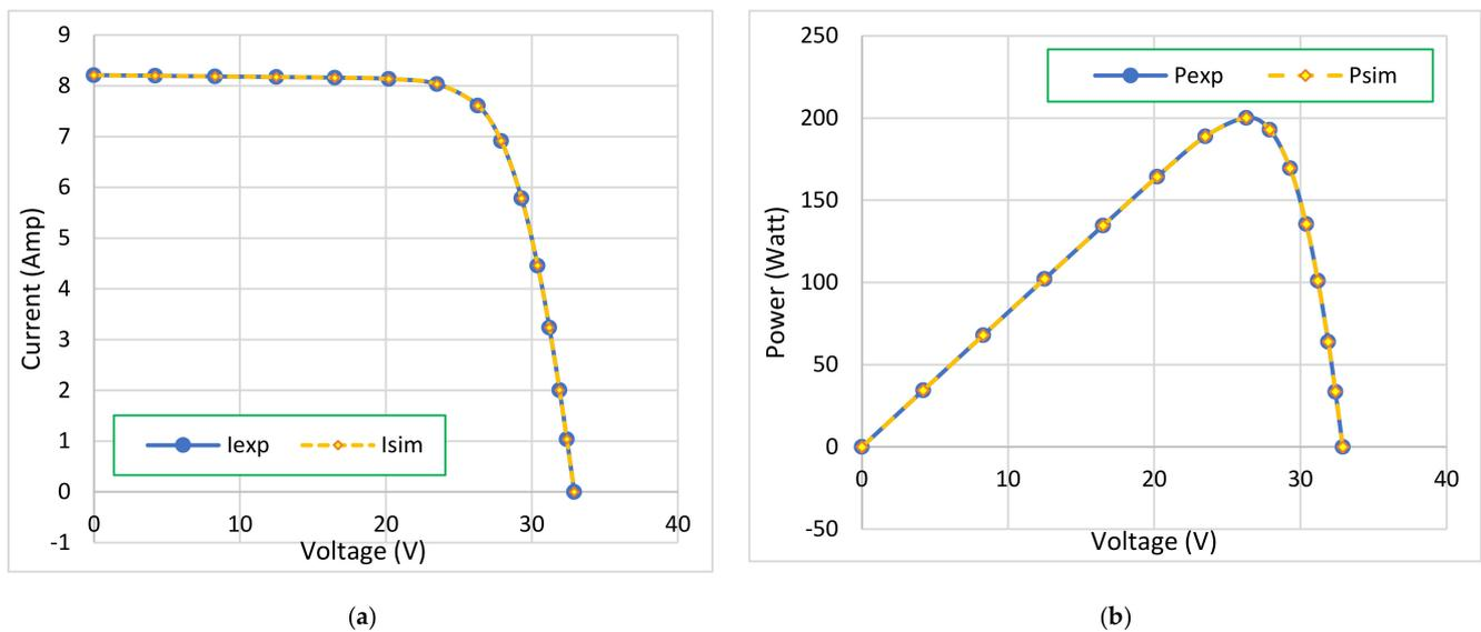
**Figure 20.** Characteristic curves for KC200GT DDM based on TFWO: (a) I–V ch/s and (b) P–V ch/s.
