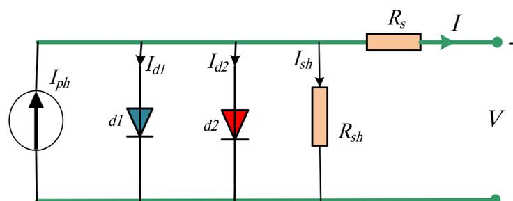
Figure 2. Double diode model (DDM) equivalent circuit.
