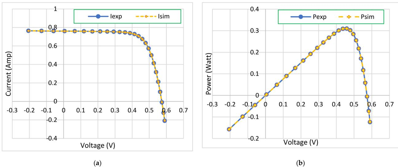
Figure 10. Characteristic curves for R.T.C. France DDM based on TFWO: (a) I–V ch/s and (b) P–V ch/s.
