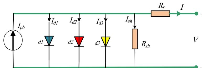
Figure 3. Three diode model (TDM) equivalent circuit.
