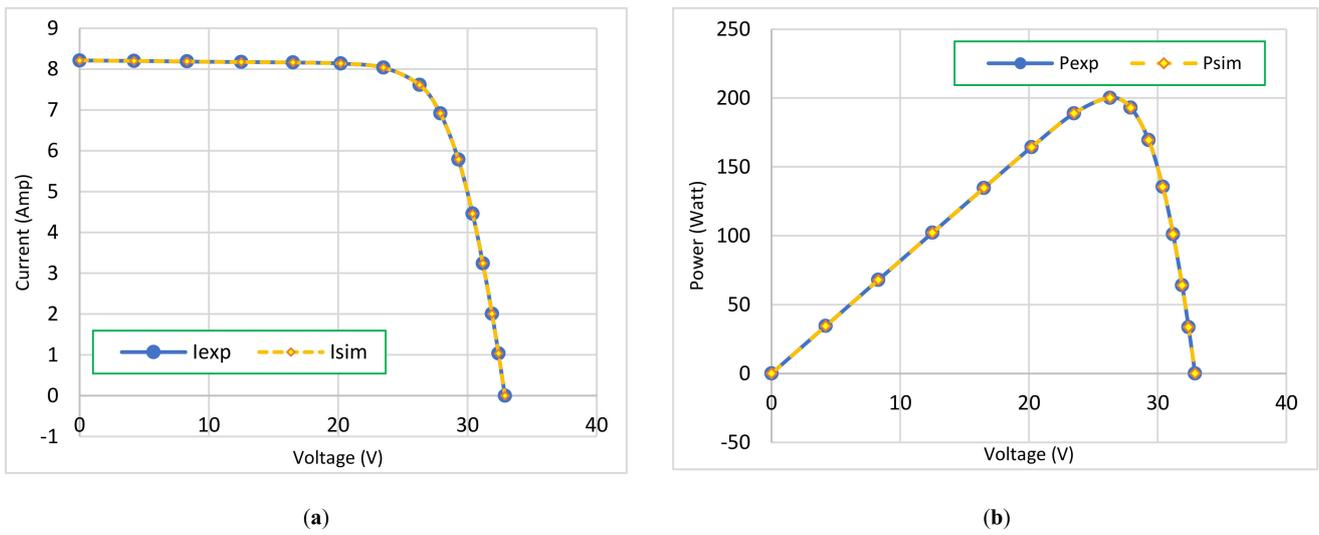
Figure 22. Characteristic curves for KC200GT TDM based on TFWO: (a) I–V ch/s and (b) P–V ch/s.
