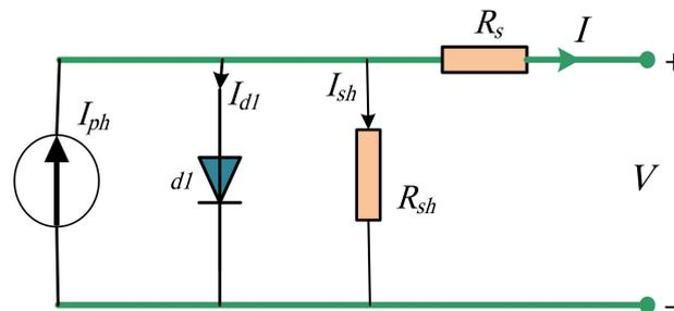
Figure 1. Single diode model (SDM) equivalent circuit.
