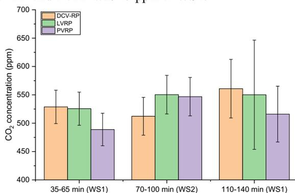
**Figure 8.** The mean CO<sub>2</sub> concentration at two workstations during sedentary periods with the three systems.
