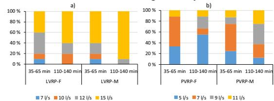
**Figure 4.** Self-controlled air flow rates from a) a low velocity unit combined with a radiant panel system (LVRP), and b) personalized ventilation combined with a radiant panel system (PVRP) adjusted by female (F) and male (M) subjects.
