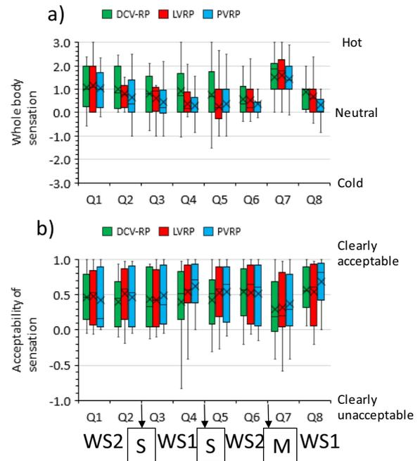
**Figure 6.** a) Whole-body thermal sensation and b) acceptability for the three systems. Questionnaires Q1, Q2, Q5 and Q6 were answered at WS2; Questionnaires Q3, Q4, Q7 and Q8 were answered at WS1. “S” refers to the slight task; “M” refers to the medium task.
