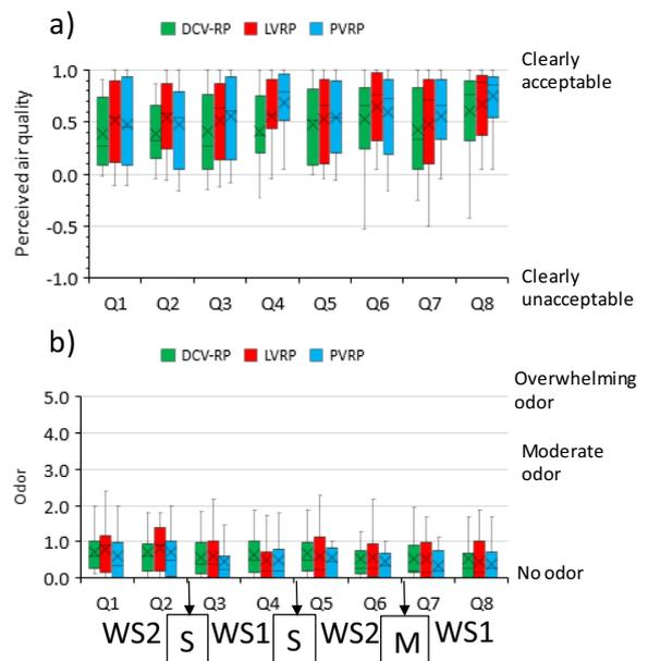
**Figure 5.** a) Perceived air quality and b) odor ratings for the three systems. Questionnaires Q1, Q2, Q5 and Q6 were answered at WS2; questionnaires Q3, Q4, Q7 and Q8 were answered at WS1. “S” refers to the slight task; “M” means medium task.
