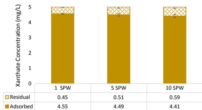
Fig. 6. Collector concentration adsorbed on chalcopyrite surface and remaining in solution.
