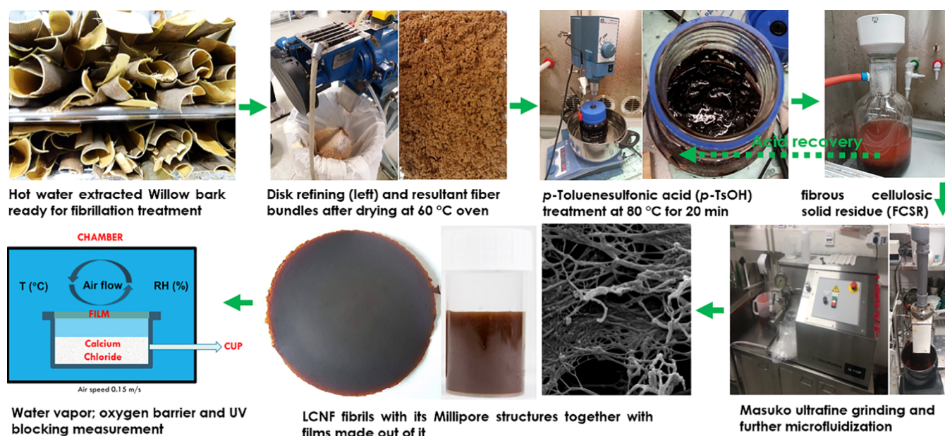
Figure 1. Experimental flow of fabricating lignin-containing cellulose nanofibrils (LCNF) and LCNF films from hot water-extracted willow bark (HWEWB), using a recyclable acid hydrotrope ( p -TsOH).
