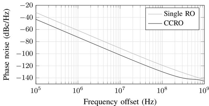
Fig. 20. Simulated phase noise of the CCRO and that of a ring oscillator with inverters of same transistor dimensions. Phase noise is reduced by more than 11 dB with CCRO.
