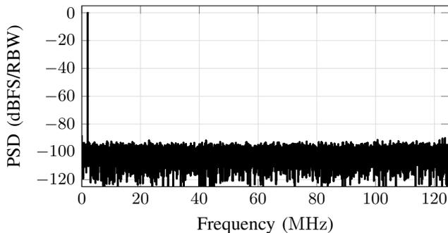
Fig. 16. Spectrum of the converter output for a single-tone test with an input frequency of 2 MHz obtained from transistor-level simulation with device noise enabled. The sample rate is 250 MHz.
