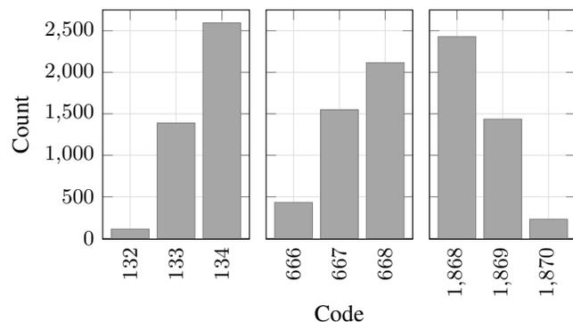
Fig. 18. Single shot precision illustrated by the histogram for low, mid, and high codes. The respective standard deviations are 0.54 LSB, 0.67 LSB, and 0.60 LSB.
