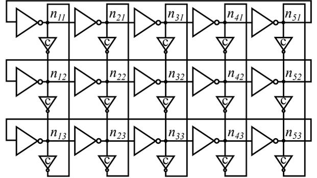
Fig. 5. A  $5 \times 3$  cyclic-coupled ring oscillator.
