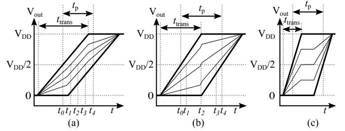
Fig. 3. Illustration of how passive/active voltage-mode interpolation fails to operate when the value of  $t_p$  exceeds the value of  $t_{trans}$  ( $F = 4$ ).
