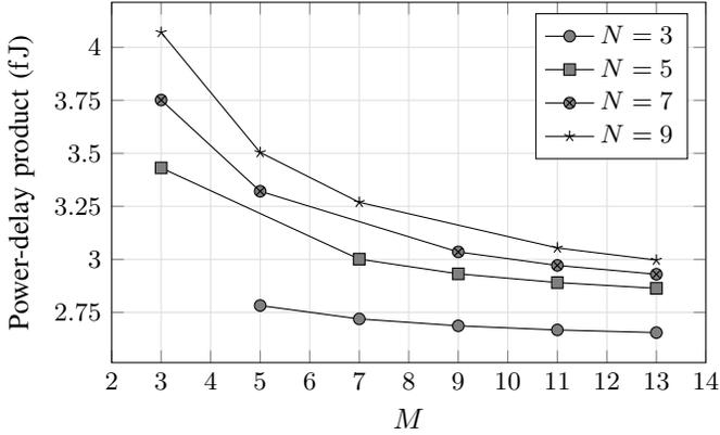
Fig. 10. Power-delay product ( $P_{\text{avg}} \times t_q$ ) of the CCROs as a function of  $M$  for different values of  $N$ .
