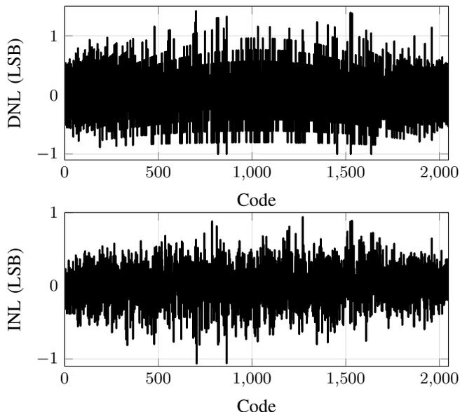
Fig. 17. DNL and INL of the converter.
