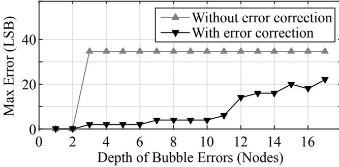
Fig. 15. Simulated demonstration of the robustness of the bubble error suppression logic to arbitrary reordering patterns as indicated by the maximum encoding error plotted against the number of taps on which the bubbles are spread, for the example of a six-bit encoder. Each data point is simulated with a large number of test vectors with random bubble patterns.
