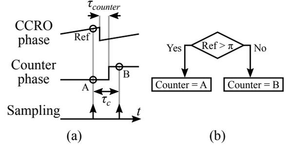
Fig. 14. Delayed double sampling of the counter phase (a) and selection logic for reliably selecting error-free counter samples (b).
