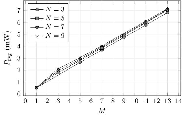
Fig. 9. Power consumption as a function of  $M$  for different values of  $N$ .
