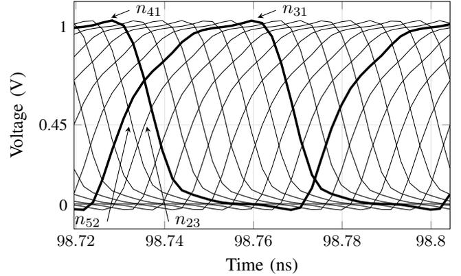
Fig. 7. Output waveform from transistor-level simulation of a  $5 \times 3$  CCRO, demonstrating a uniform sub-gate-delay phase division at an effective switching threshold of 0.45 V. Two adjacent transitions of a horizontal oscillator are highlighted with bold lines, showing the two uniformly spaced additional transitions between them.
