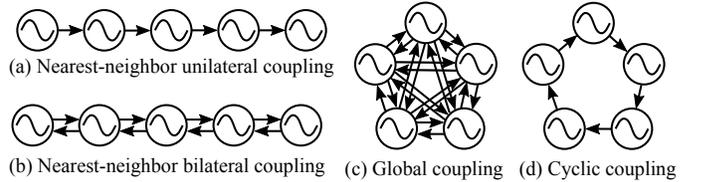
Fig. 4. Various configurations of coupled oscillators.
