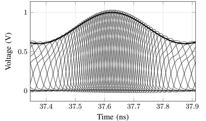
Fig. 12. Operation of a  $5 \times 3$  CCRO as a supply controlled VCO, enabling its use in VCO-based ADCs.
