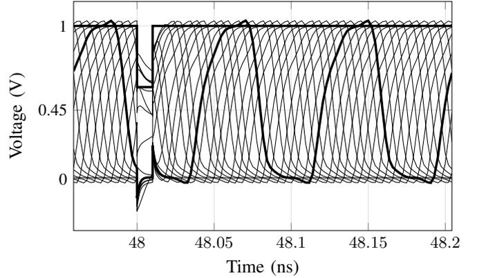
Fig. 11. Response of a CCRO to a 0.4 V drop in power supply for 10 ps, demonstrating the resilience of the phase relationship among the nodes to supply fluctuations. The uniform spacing of the transitions is restored within a couple of cycles. The supply voltage and one node voltage are highlighted with bold lines.
