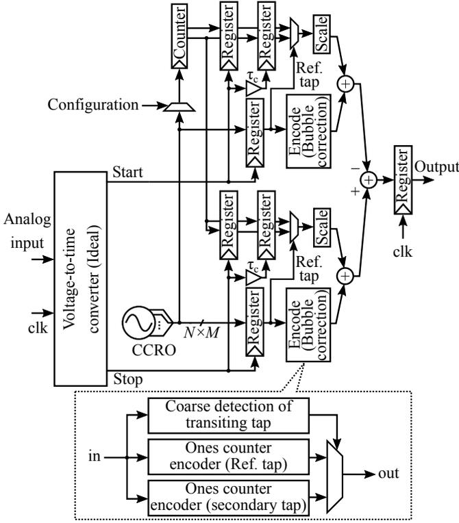
Fig. 13. Implemented circuit and the simulation set up.
