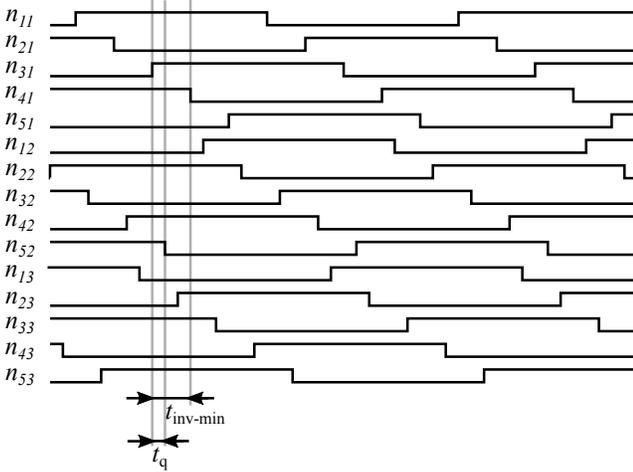
Fig. 6. The waveform at the multi-phase output of the CCRO in Fig. 5 for the mode with  $\psi = 120^\circ$ .  $M = 3$  yields a factor-of-three improvement in phase resolution.
