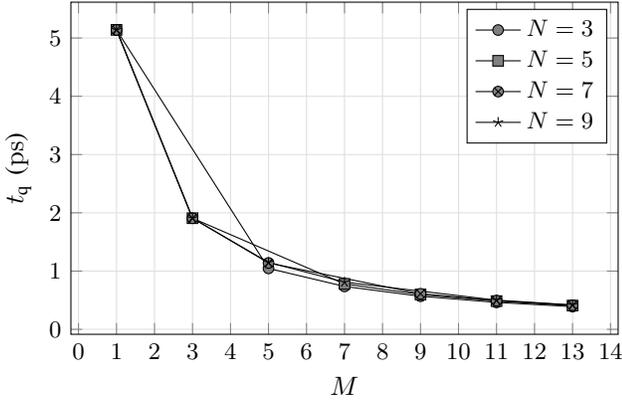
Fig. 8. Time resolution as a function of  $M$  for different values of  $N$ .  $M = 1$  corresponds to a regular ring oscillator with same transistor dimensions and similar loading conditions as a CCRO.
