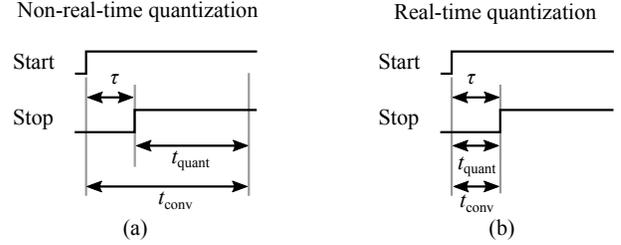
Fig. 2. Two types of time-to-digital converters: (a) non-real-time quantizing converters which quantize the target delay  $\tau$  after the arrival of the stop signal and (b) real-time quantizing converters that quantize the delay between the start signal and the stop signal. Real-time converters are desired since they allow higher sample rates and conversion bandwidth.
