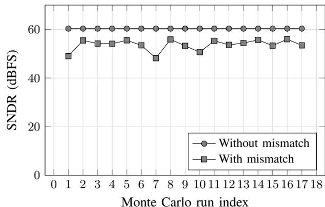
Fig. 19. Monte Carlo simulation result demonstrating the variation of performance in the presence of process mismatch.
