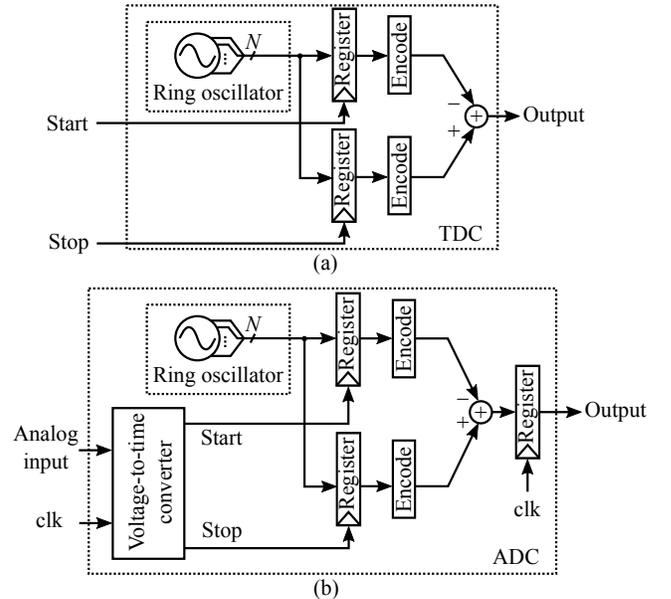
Fig. 1. Examples of oscillator-based data converters: (a) a time-to-digital converter, and (b) a time-domain ADC consisting of a voltage-to-time converter and a time-to-digital converter
