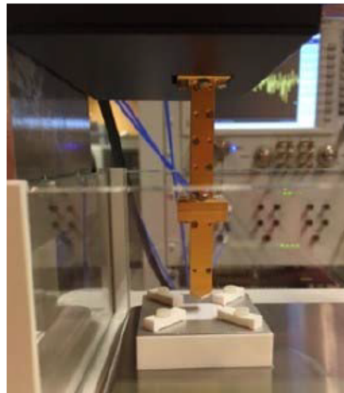
Fig. 1 Experimental setup: millimeter-wave module and sample placed on the scale.
