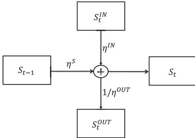
Fig. 2. Storage level end of period is determined based on previous storage level and charge & discharge during period  $t$  using corresponding efficiency ratios.
