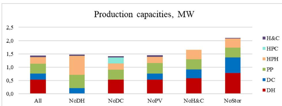
Fig. 7. Optimized heat and cooling production capacities in scenarios.
