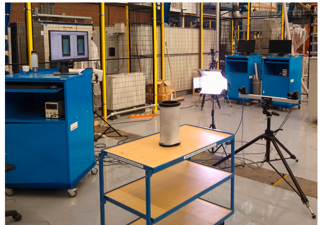
Fig. 4. Experimental setup for the DIC measurements.
