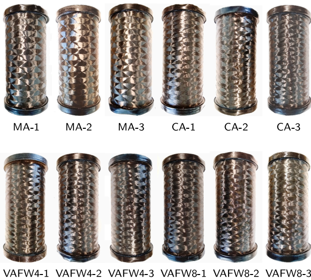
Fig. 2. Filament-wound cylinders used in the imperfection measurements.
