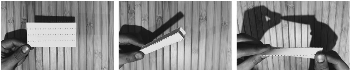
Figure 1: The generation principles of the shape through a paper model: (a) a piece of paper with four segments, (b) folding a square cross-section tube, (c) cross-wisely connecting the tube's short edges to restrain the 1-DOF-mechanism
