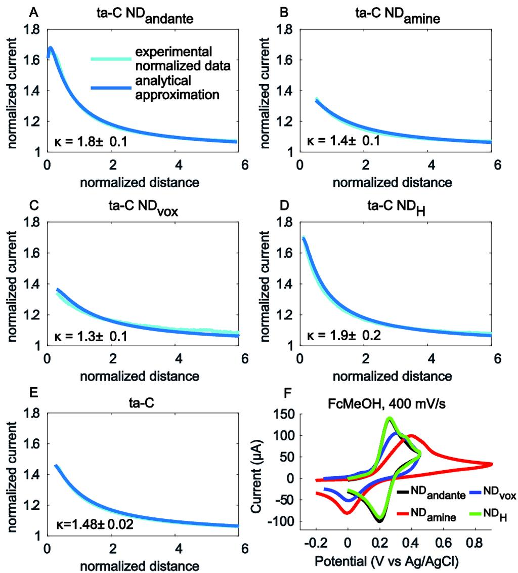
Figure 2: FcMeOH electrochemistry on nanodiamonds. The approach curves recorded in 1 mM FcMeOH with 10  $\mu\text{m}$  Pt tip on (A) ND<sub>andante</sub>, (B) ND<sub>amine</sub>, (C) ND<sub>vox</sub>, (D) ND<sub>H</sub> and (E) the reference ta-C. (F) Cyclic voltammetry of 1 mM FcMeOH on different spray-coated ND functionalities.
