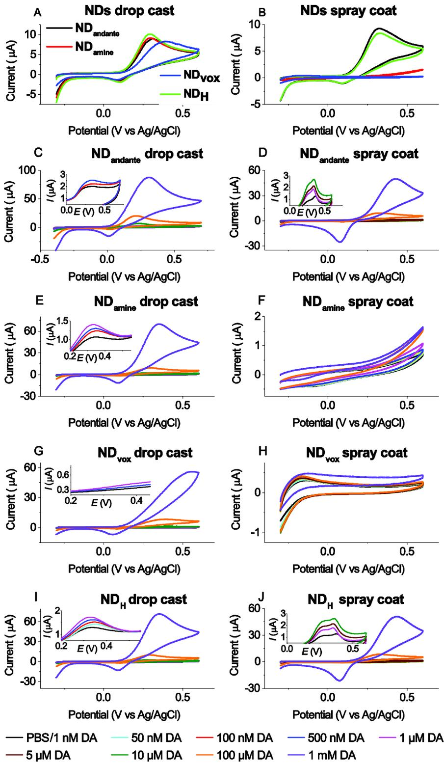
Figure 4: Dopamine detection using nanodiamonds. Left column shows the dopamine detection on drop-casted nanodiamonds and right column on spray-coated nanodiamonds. Cycling speed 50 mV/s.
