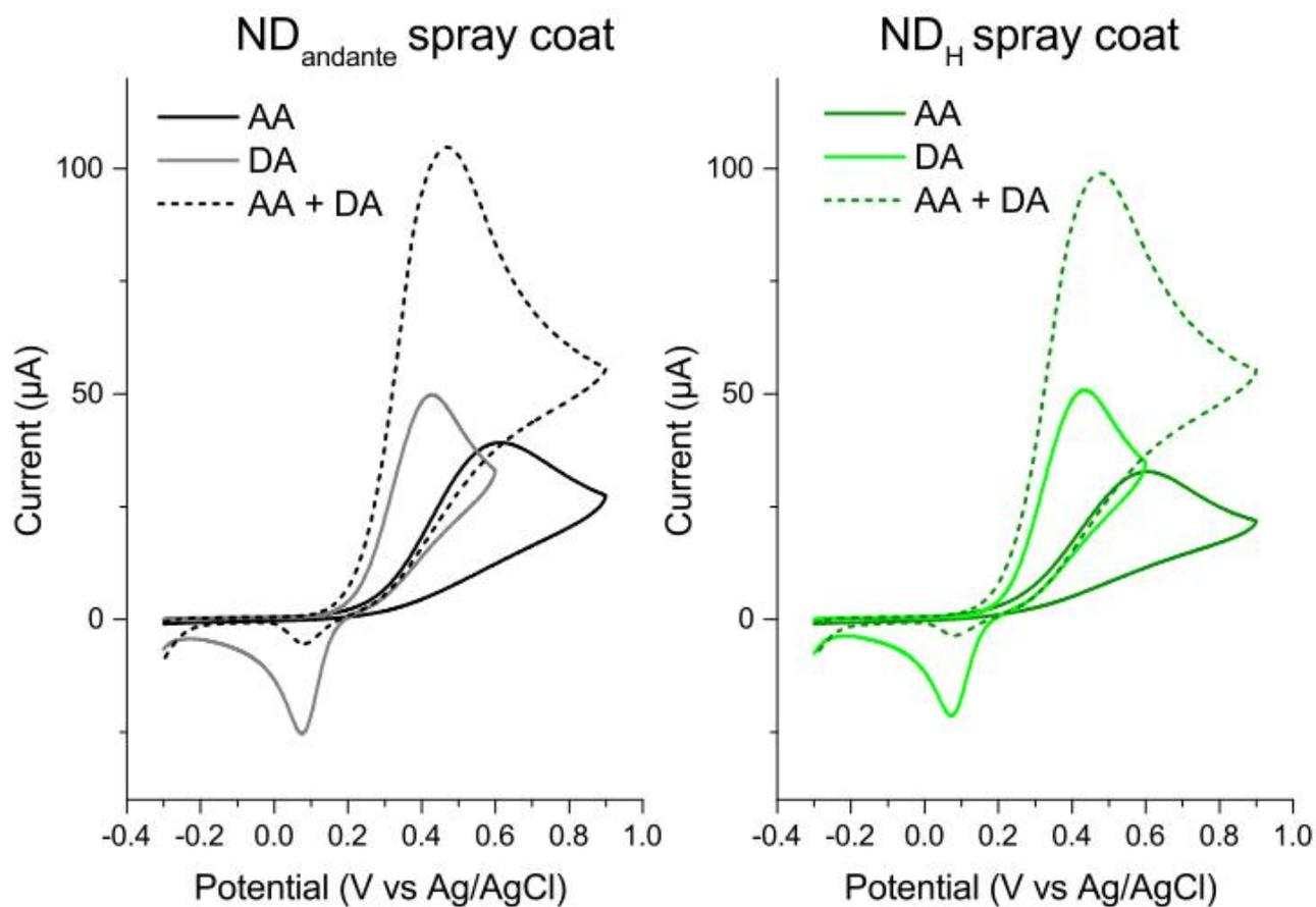
Figure 5: Selectivity of spray-coated nanodiamonds. Measurements were done in 1 mM dopamine and 1 mM ascorbic acid, both separately and together.
