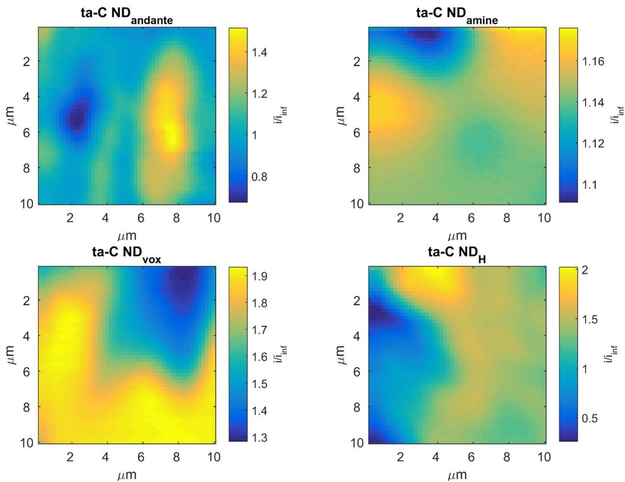
Figure 3: Scanning electrochemical microscopy images recorded in feedback mode on nanodiamond surfaces using  $2\ \mu\text{m}$  Pt electrode.
