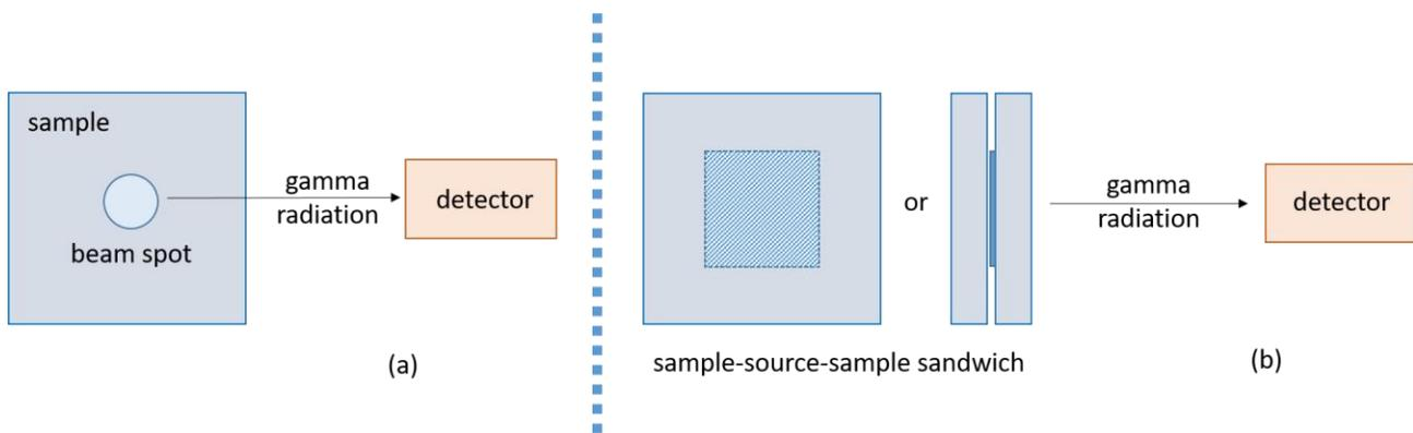
Figure 1. (a) Typical measurement geometry in a slow positron beam. The detector is aligned perpendicular to the incoming beam and hence to the surface normal, i.e., the direction of the measurement is along a crystal orientation within the surface plane of the sample. (b) Typical measurement geometry in a fast positron experiment. The detector is placed either in a similar orientation as in the slow positron beam experiment, or along the surface normal of the samples.
