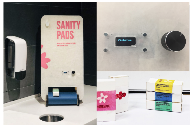
Figure 6: The final prototype of the vending machine, a close up of the display it had on top and the boxes that contained the sanity pads.
