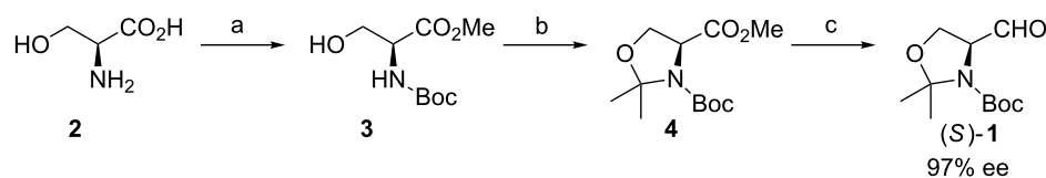
Scheme 4: The Koskinen procedure for the preparation of Garner's aldehyde. (a) i) \text{AcCl} , \text{MeOH} , 0 °C \rightarrow 50 °C (99%); ii) (\text{Boc})_2\text{O} , \text{Et}_3\text{N} , \text{CH}_2\text{Cl}_2 , 0 °C \rightarrow rt (95–99%); (b) \text{Me}_2\text{C}(\text{OMe})_2 , \text{BF}_3 \cdot \text{Et}_2\text{O} , \text{CH}_2\text{Cl}_2 , rt (86%, after high vacuum distillation); (c) DIBAL-H, toluene, –84 °C ( \text{EtOAc}/\text{N}_2 bath) (82–84%, after high vacuum distillation).
