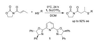
A Sc complex of (4S,5S)-diphenyl PYBOX **1** was found to serve as a catalyst for the asymmetric conjugate addition reactions between various thiols and 3-crotonoyl-2-oxazolidinone, affording the corresponding adducts in good yields and high enantioselectivies (up to 92% ee). A new improved method for making (4S,5S)-diphenyl PYBOX is presented.
