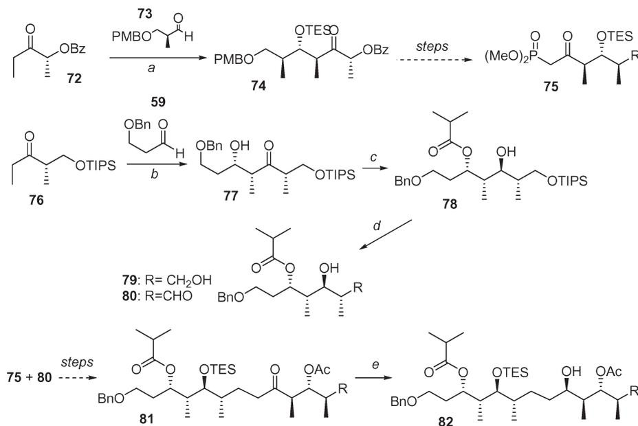
**Scheme 9** a 1. (c-Hex)<sub>2</sub>BCl, Me<sub>2</sub>NEt, Et<sub>2</sub>O, 0 °C, 1 h, then -78 °C, **73**, to >-20 °C, 16 h; 2. TESOTf, 2,6-lutidine, CH<sub>2</sub>Cl<sub>2</sub>, -78 °C, 2 h; b Sn(OTf)<sub>2</sub>, Et<sub>3</sub>N, CH<sub>2</sub>Cl<sub>2</sub>, **59**, -78 °C, 2 h; c isobutyraldehyde, SmI<sub>2</sub>, THF, 0 °C, 2.5 h; d 1. HF·pyridine, THF, rt, 7 h; 2. cat. TEMPO, PhI(OAc)<sub>2</sub>, rt, 2 h; e SmI<sub>2</sub>, CH<sub>3</sub>CHO, THF, -5 °C, 2.5 h.
