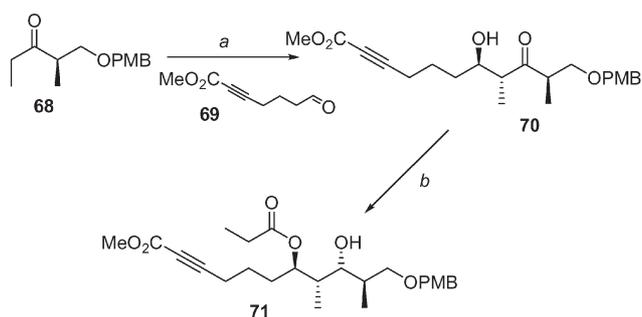
**Scheme 8** a (c-Hex)<sub>2</sub>BCl, Et<sub>3</sub>N, Et<sub>2</sub>O, 0 °C, 1 h, then -78 °C and **69** to >-20 °C, 12 h, oxidative work-up; b SmI<sub>2</sub>, EtCHO, THF, 0 °C, 15 min, then **70**, 0 °C, 2 h.
