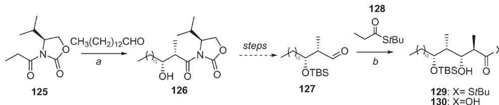
Scheme 15 *a* *n*-Bu<sub>2</sub>BOTf, Et<sub>3</sub>N, CH<sub>2</sub>Cl<sub>2</sub>, 0 °C, 0.5 h, then -78 °C, tetradecanal, 12 h; *b* **128**, (Chx)<sub>2</sub>BCl, Et<sub>3</sub>N, CH<sub>2</sub>Cl<sub>2</sub>, 0 °C, 2 h, then -78 °C, **127**, 12 h, oxidative work-up.
