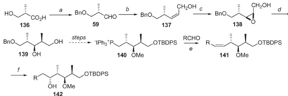
**Scheme 17** a 1.  $\text{PhCH}_2\text{OC}(\text{=NH})\text{CCl}_3$ ,  $\text{CF}_3\text{SO}_3\text{H}$ ; 2.  $\text{LiAlH}_4$ ; 3. Swern oxidation; b 1.  $(\text{CF}_3\text{CH}_2\text{O})_2\text{P}(\text{=O})\text{CH}_2\text{CO}_2\text{Me}$ ,  $\text{KN}(\text{TMS})_2$ , 18-Crown-6; 2. DIBAL-H; c MCPBA; d  $\text{Me}_2\text{CuLi}$ ; e *n*-BuLi; f  $\text{B}_2\text{H}_6$ ,  $\text{H}_2\text{O}_2$ .
