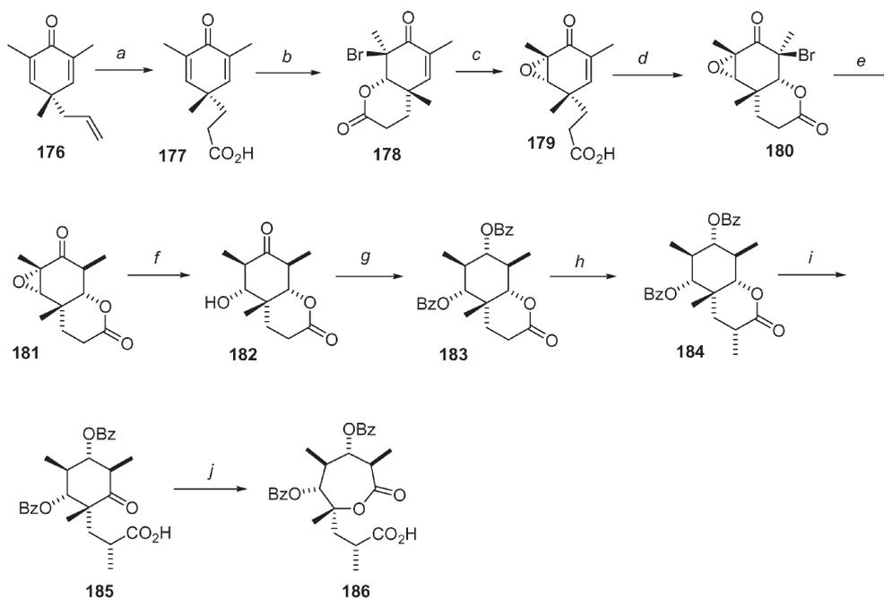
**Scheme 23** a 1.  $B_2H_6$ , THF, 0–10 °C; 2. Jones chromic acid, 0––10 °C; b  $Br_2$ , KBr,  $H_2O$ ; c aq. KOH, THF; d  $Br_2$ , KBr,  $H_2O$ ; e  $Bu_3SnH$ , AIBN, PhH; f Al/Hg, THF,  $H_2O$ , 0 to –10 °C; g 1.  $H_2$ , Raney Ni, DME, –20 °C; 2. BzCl, pyridine; h LDA, THF, –78 °C, then MeI, HMPA, –78 °C to >–45 °C; i 1. LiOH,  $H_2O$ ; 2.  $CrO_3$ ,  $H_2SO_4$ , acetone, –10 °C; j  $MeCO_3H$ , EtOAc, 55 °C.
