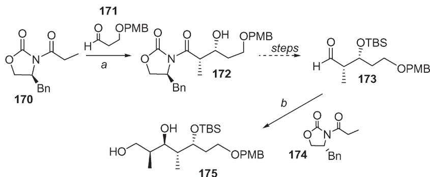
**Scheme 22** a *n*-Bu<sub>2</sub>BOTf, CH<sub>2</sub>Cl<sub>2</sub>, Et<sub>3</sub>N, -5 °C, then -78 °C, **171**; b 1. **174**, *n*-Bu<sub>2</sub>BOTf, CH<sub>2</sub>Cl<sub>2</sub>, Et<sub>3</sub>N, -5 °C, then -78 °C, **173**; 2. LiBH<sub>4</sub>, THF–MeOH, 0 °C.
