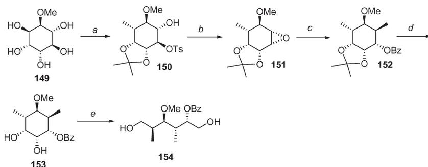
**Scheme 19** a 1. ref. 36; 2.  $\text{Bu}_2\text{SnO}$ , MeOH, reflux, then TsCl, DMAP; 3. 1,4-dioxane, rt; b MeONa, MeOH, reflux; c 1.  $\text{Me}_3\text{Al}$ ,  $\text{CH}_2\text{Cl}_2$ : hexanes, rt; 2. BzCl, pyridine, DMAP, rt; d 10-camphorsulfonic acid, MeOH, rt; e  $\text{NaIO}_4$ , acetone- $\text{H}_2\text{O}$ ,  $0^\circ\text{C}$ , then  $\text{NaBH}_4$ , MeOH,  $0^\circ\text{C}$ .
