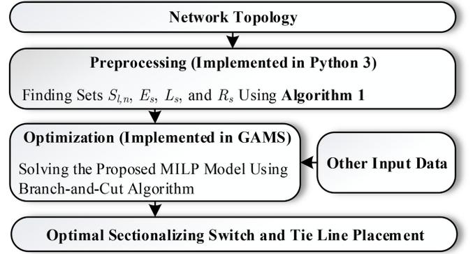
Fig. 3. Flowchart of the implementation procedure.
