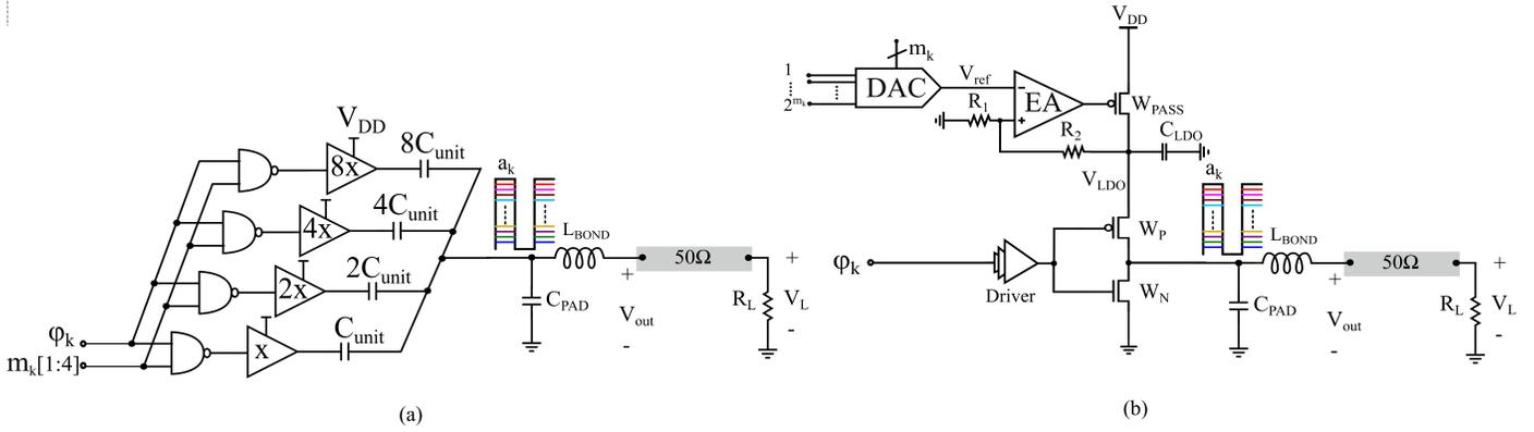
Fig. 4. (a) A 4-bit binary weighted SCPA structure with class-D PA units (b) A LDO based supply scaling topology for class-D PA
