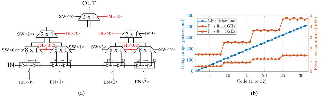
Fig. 3. (a) Optimized phase tuning architecture (b) An optimized 5-bit delay line characteristics vs phase scaling codes.
