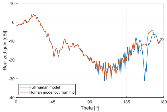
Fig. 2. Comparison of realized gain of an antenna element, simulated with truncated and full-sized numerical human models; the gain patterns represent \phi = 270^\circ cut.
