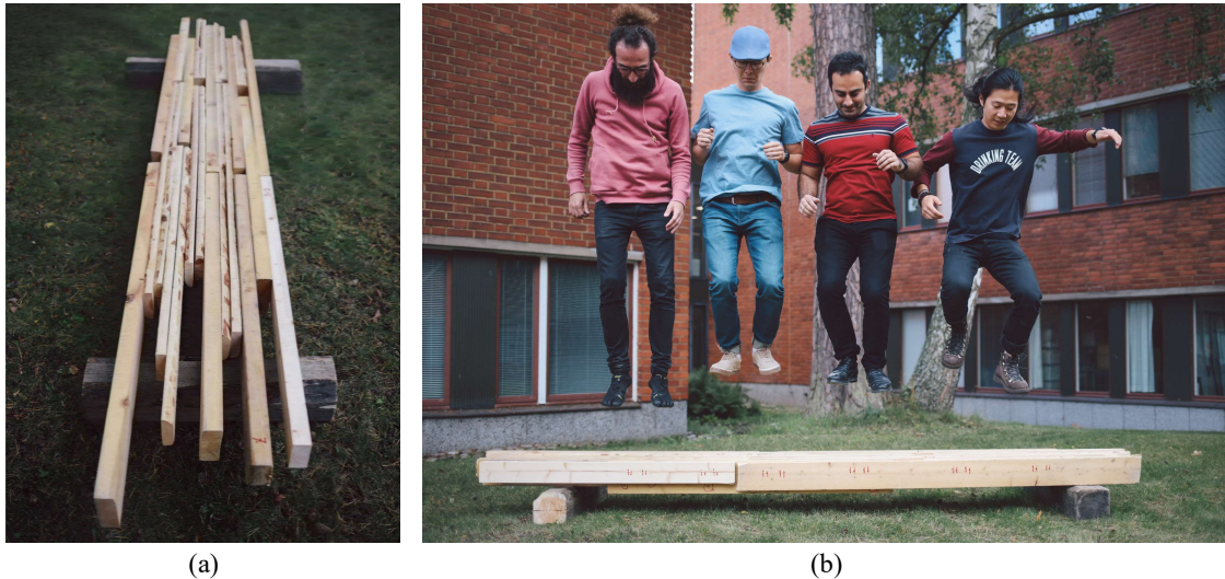
Figure 6: Prototype-structure: (a) a simply supported NLT deck realized by salvaged timber and wooden nails; (b) a loading test on the structure including its prototypical use.
