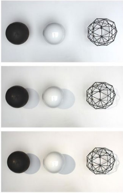
Figure 5. Light modelling experiments with different ratio of diffuse and direct light. From the top and down the electrical light setting referring to sky type 3, 8 and 13. Photo: Michael Cleary and Mihkel Pajuste.
