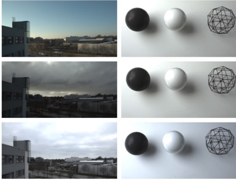
Figure 4. Different sky conditions, from the top and down referring to the daylight inflow with respectively CIE sky types 13, 3 and 8 and to the right photo illustrating how the different daylight situations affect light modelling qualities of the spheres. Photo: Mihkel Pajuste.
