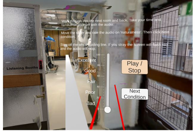
Fig. 6. Screenshot of the virtual reality visuals, displaying the control panel and instructions for the test, as well as a white line designating the allowed path to follow. Should the participant stray more than 25 cm from the guiding line in the X or Z axis, the screen flashes red and the audio cuts out.
