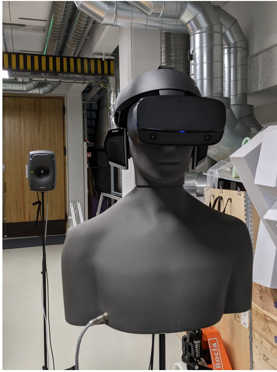
(a) Cortex dummy head wearing the Oculus Rift S and Mysphere 3.2 headphones
