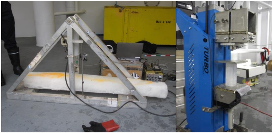
Figure 1. Test setup for the bending strength (left) and compressive strength (right) of ice measurements (Suominen, et al., 2013).
