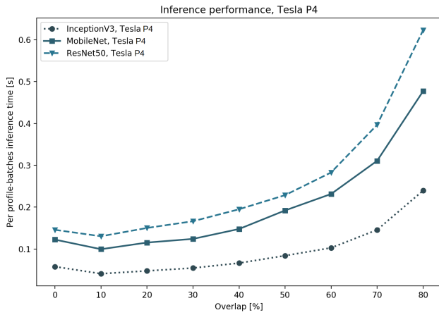
Fig. 5: Mean inference times for different amount of profile batches (overlap values) using the three CNN models on NVidia Tesla P4 GPU.
