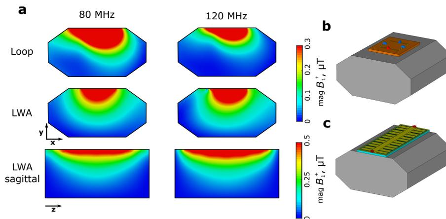
**Figure 2.** (a) Simulated  $B_1^+$  magnitude distributions normalized by square root of accepted power. (b) CST model of investigated coils, loaded with homogeneous phantom.
