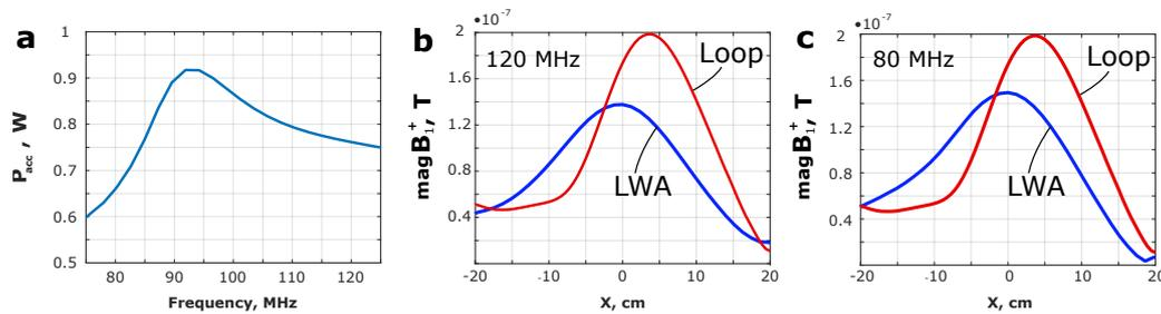
**Figure 3.** Results of numerical simulations: (a) Simulated power, dissipated in the phantom, over the wide frequency range for leaky-wave antenna. (b) Simulated  $B_1^+$  magnitude at the 10 cm depth in the phantom for the LWA and loop coil at 120 MHz. (c) Simulated  $B_1^+$  magnitude at the 10 cm depth in the phantom for the LWA and loop coil at 80 MHz.
