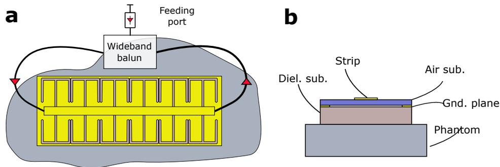
**Figure 1.** Schematic layout of the proposed leaky-wave antenna placed over a homogeneous phantom: (a) top view; (b) side view
