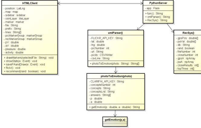
Fig. 1: UML class diagram: System architecture and structure
