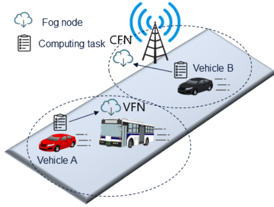
Fig. 1: An application Scenario of VFC, where Vehicle A offloads its task to a VFN carried by a bus and Vehicle B offloads its task to a CFN co-located with a cellular base station.
