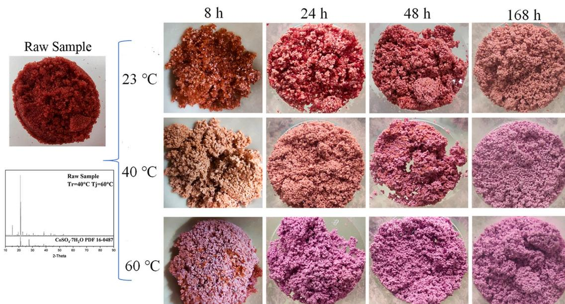
Fig. 12. Sample images with different drying times at various drying temperatures.
