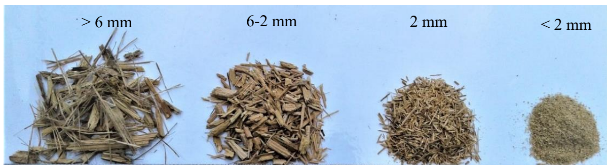
148 149 Figure 1. Prepared date palm fronds feedstock at various particle size ( d_p ) for air gasification.
