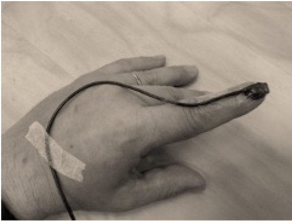
FIGURE 3 | A typical setting in corticokinematic coherence studies (42–44) with a lightweight accelerometer (ADXL335; Analog Devices Inc, Norwood, MA) attached on the finger nail to pick up hand movements. Note that flexible cable allows natural hand movements.
