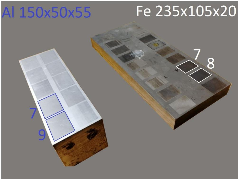
**Figure 4: Measured samples, where aluminium is on the left-hand side, marked in blue, while the steel sample is on the right-hand side, marked in white. The burnished areas are highlighted and numbered with corresponding colour. The dimensions of the pieces are given in mm. All the burnished areas are equally large (30 mm x 20 mm).**
