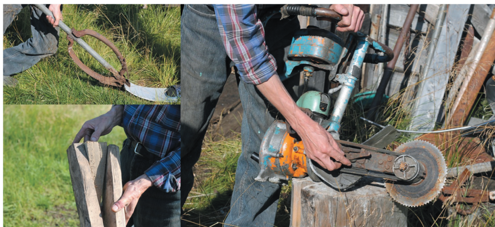
Figure 5. For working with the four-millimetre sheet metal, the local boat-makers crafted (top left) a bender ( zagibulina ) for shaping the beak and sides of the boat; (bottom left) a wooden vice for clamping workpieces in place; and (right) a new metal cutter for the ‘Druzhba’ gasoline chainsaw. Photos by Alexandra Raeva, August 2018.
