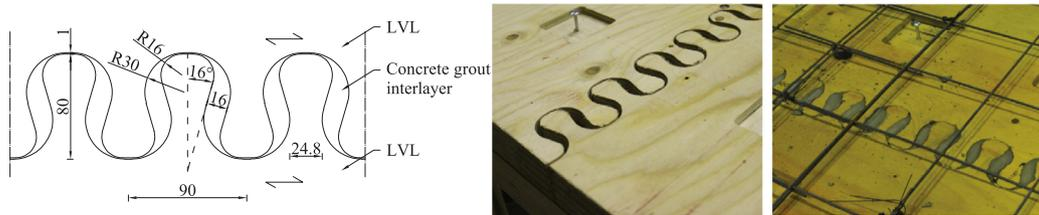
Fig. 2. Geometry of the dovetail joint with nominal dimensions in [mm] and photos of the joint in Plate 1 before and after casting the interlayer.
