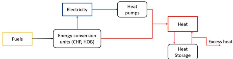
Fig. 1. Schematic diagram of the DH model by EnergyPRO.
