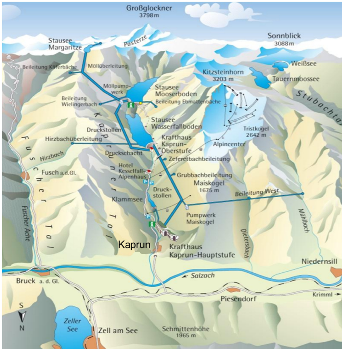
Fig. 1. Conventional hydropower in steep mountains. Kaprun hydropower and pumped storage plant in Austria. The plant consists of high dams and tunnels to increase the catchment area of the plant and to connect to the Salzach River and the lower reservoir Zeller See.
