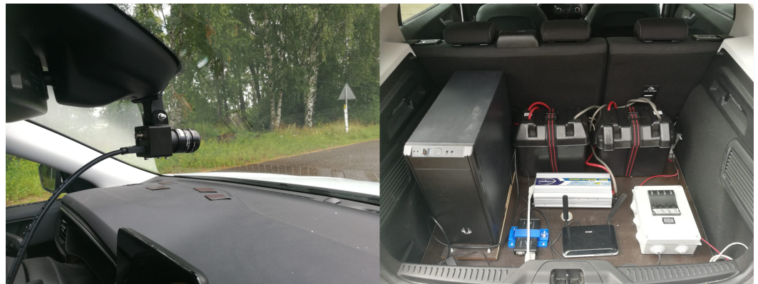
Figure 2. Hardware installations on the test vehicle. The windshield camera installation on the (left) and computational power with accessories on the (right).
