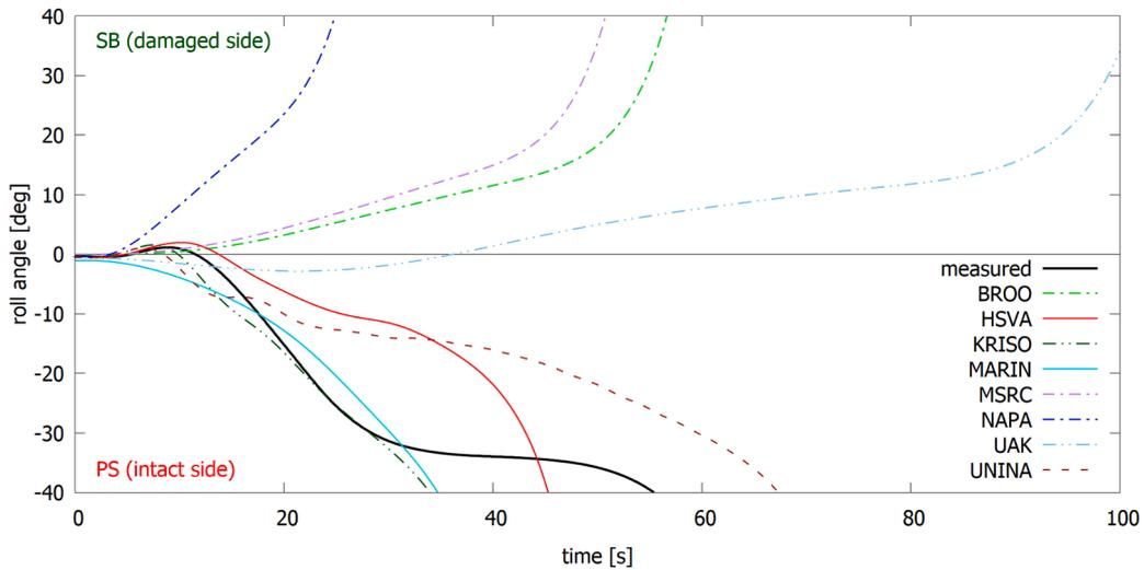
Fig. 10. Comparison of roll angle for transient flooding Case 1b with capsizing.
