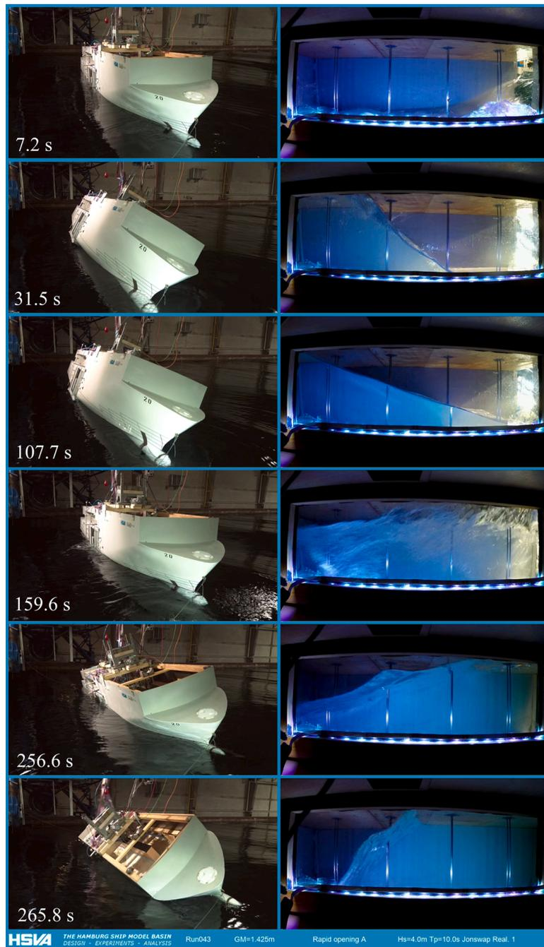
**Fig. 14.** Video captures showing the floating position and flooding of the “blue compartment” R1 in transient flooding in beam seas, with small initial heel away from the damage Case 2b, time stamps in full scale.
