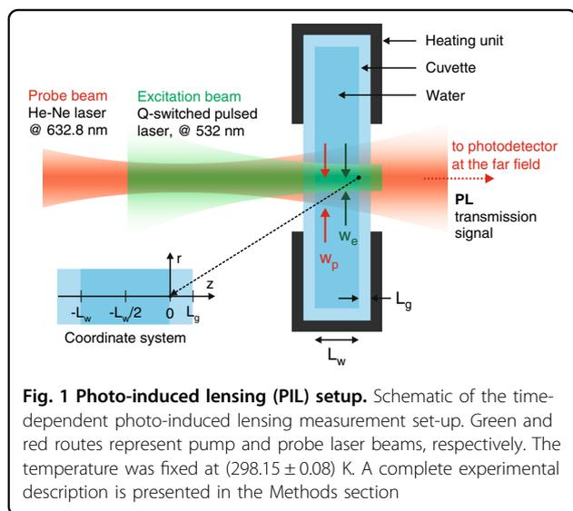
forces in addition to a small heat deposition. Nonlinear optical Kerr effect is also observed during the pulse duration. A low-irradiance laser beam traverses the sample thus probing the induced effects. The intensity of the probe beam is monitored in the far field by a fast photodetector (see Methods).
