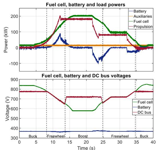
Figure 6: Power and voltage waveforms of the proposed system during normal operation.
