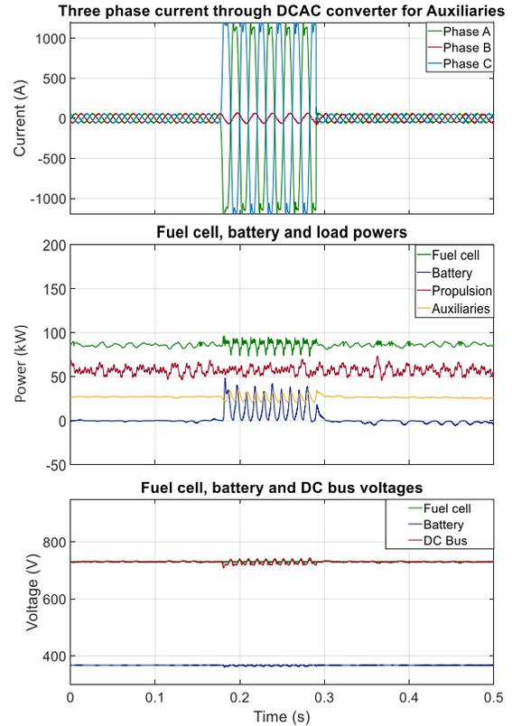
Figure 8: System behavior during a phase-to-phase short circuit in the AC network. Short circuit occurs between phases A and C
