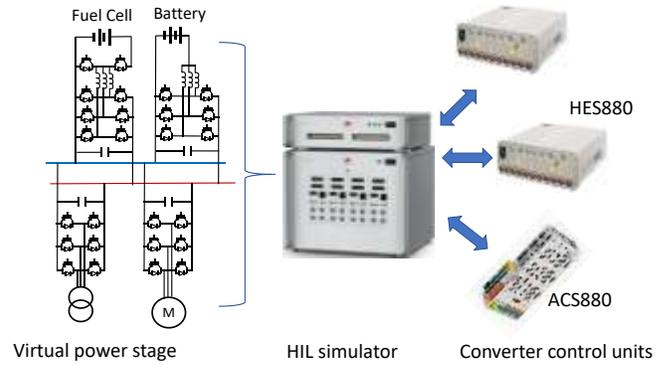
Figure 5: A HIL test setup consisting of two FC units, a battery unit, a propulsion motor unit and an auxiliary load supply unit.
