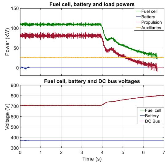
Figure 10: System behavior following a failure in the battery system.
