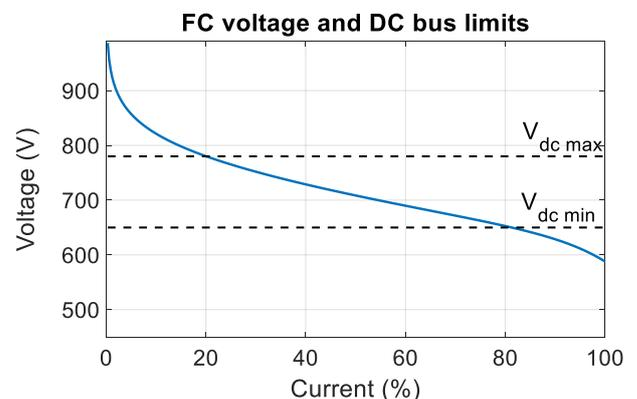
Figure 2: Fuel cell voltage as function of current in percentage of fuel cell nominal current. The  $V_{dc\_min}$  and  $V_{dc\_max}$  are the minimum and maximum DC bus voltages, respectively.
