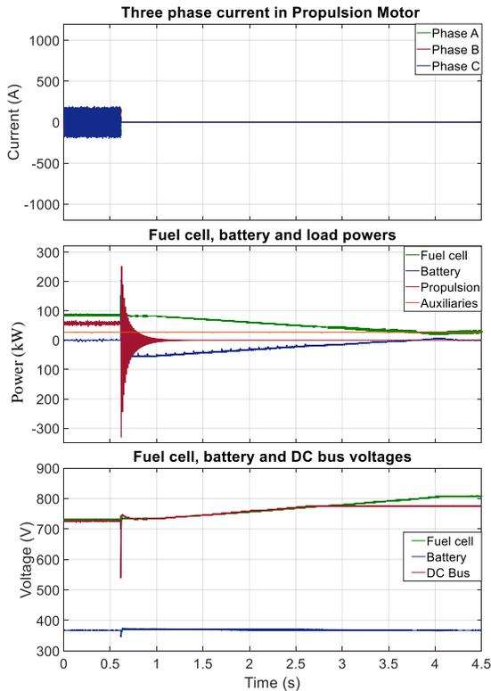
Figure 9: System behavior during a phase-to-phase short circuit in the propulsion motor terminals.
