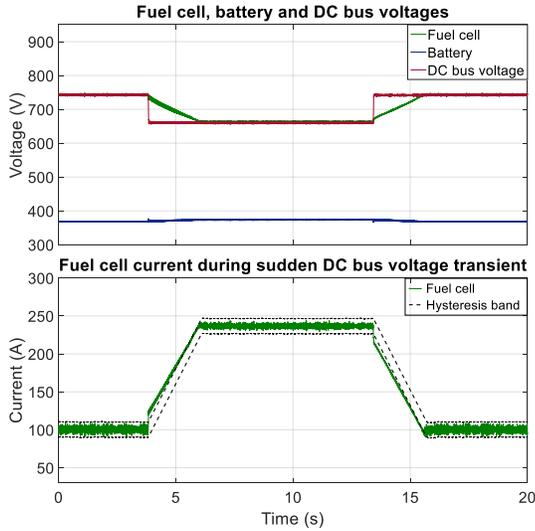
Figure 7: Fuel cell current behavior in the Freewheel mode during a sudden DC bus voltage transient.
