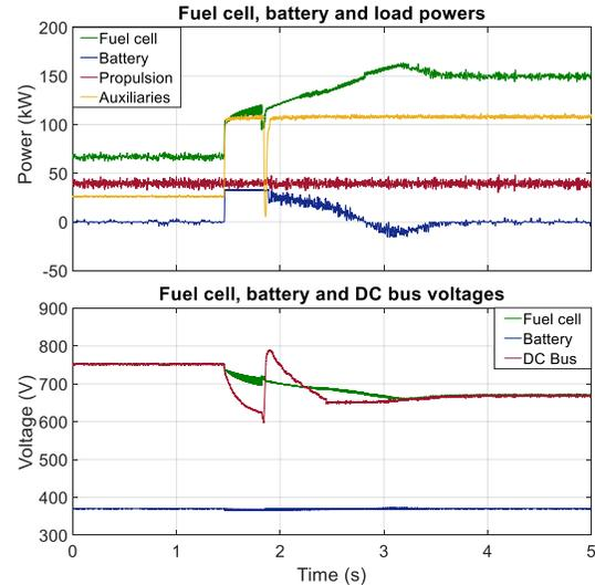
Figure 12: System behavior during a DC bus undervoltage.
