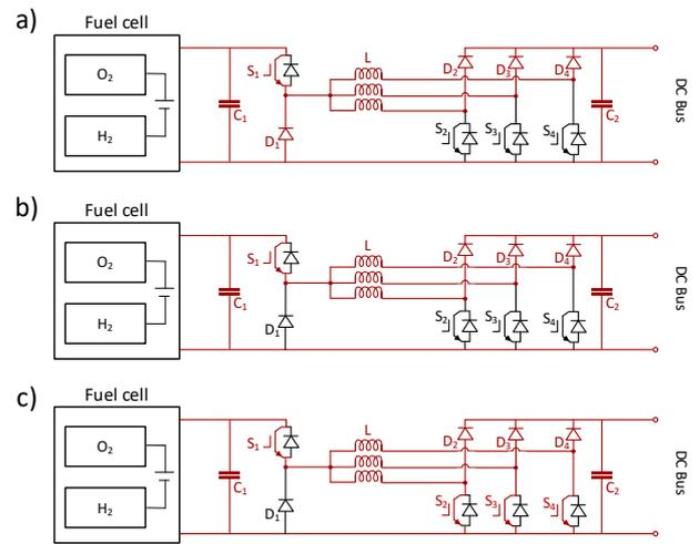
Figure 3: Operation of unidirectional buck-boost converter in a) Buck mode, b) Freewheel mode and c) Boost mode. The red color is used to highlight which components are in use in the respective modes.
