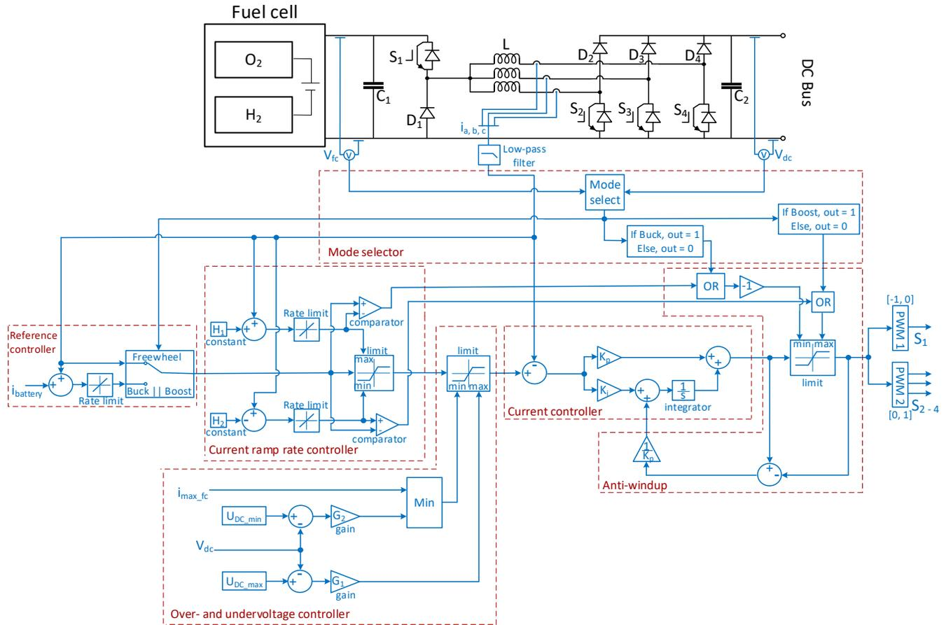
Figure 4: A control diagram for fuel cell DC/DC converter operating in a system utilizing the Variable DC approach. The output of PWM 1s is used to control switch  $S_1$ , whereas outputs of PWM2 are used for switches  $S_2 - S_4$ . In the figure,  $O_2$  and  $H_2$  refer to oxygen and hydrogen, respectively,  $D_1 - D_4$  refer to diodes,  $C_1$  and  $C_2$  refer to capacitors and  $L$  refers to inductor.
