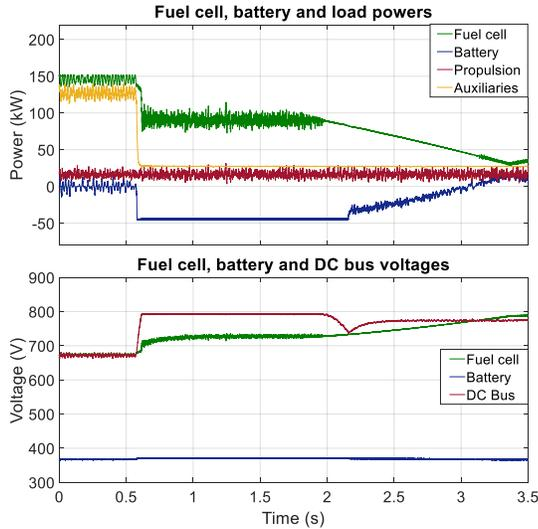
Figure 11: System behavior during a DC bus overvoltage.
