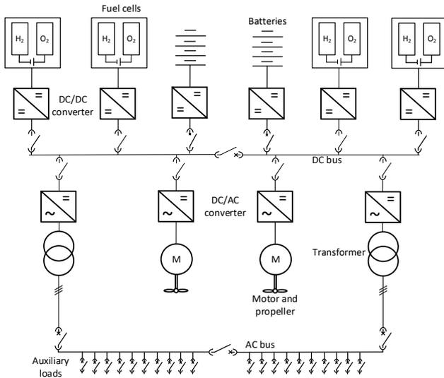
Figure 1: A generic marine power system powered by fuel cells and batteries. The auxiliary loads comprise all onboard loads other than propulsion (e.g., lighting, navigation equipment and heating and air conditioning)
