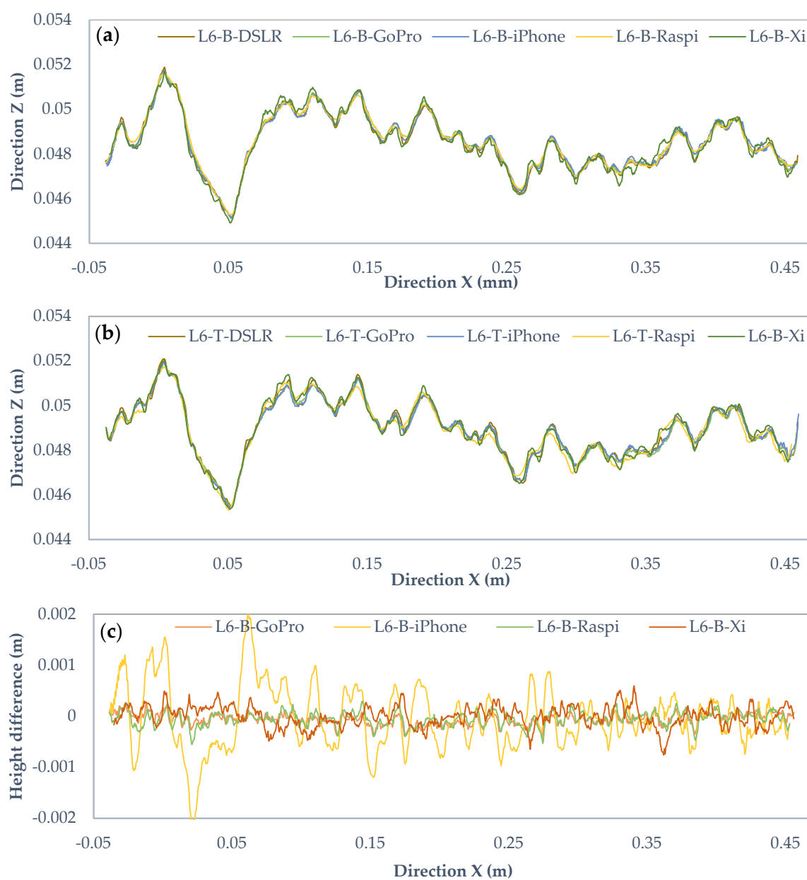
Figure 14. Comparison of the Canon EOS 5DS R DSLR and low-cost camera profiles with 0.25 mm rasterization grid interval. (a) Original profiles of bottom surface, (b) top surface, (c) height differences of bottom profiles, and (d) top profiles.
