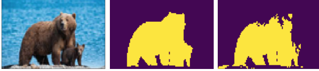
Fig. 4: Image Segmentation: The left plot is the original image, the middle one is the segmentation result from Algorithm 2, the right one is the result from spectral clustering.
