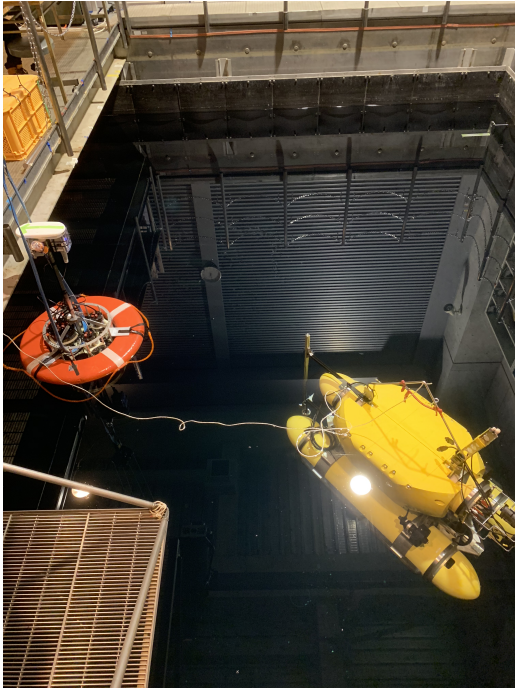
Fig. 2. Water tank experiments. The AUV Tri-TON (yellow) and the autonomous surface vehicle BUTTORI (orange) are deployed in the water tank.
