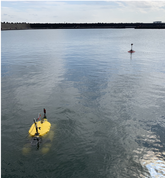
Fig. 4. Sea experiments at Hiratsuka Port. The AUV Tri-TON (yellow) and the autonomous surface vehicle BUTTORI (orange) are deployed in the sea environment.
