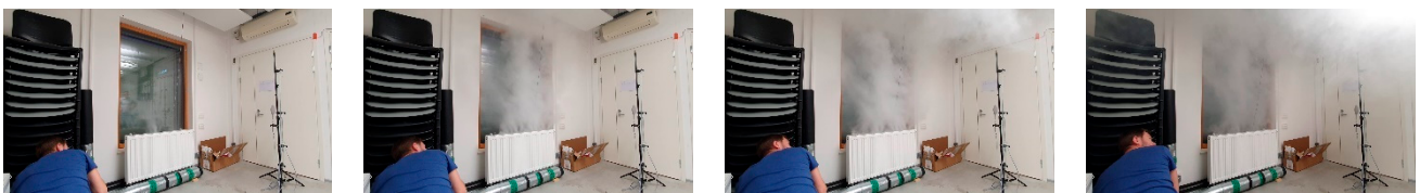
Figure 17. Air circulation pattern of radiators HIGH. Periodic snapshots every 5 s.
