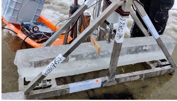
Figure 1. An ex-situ 3-point bending test (Suominen, et al., 2021).
