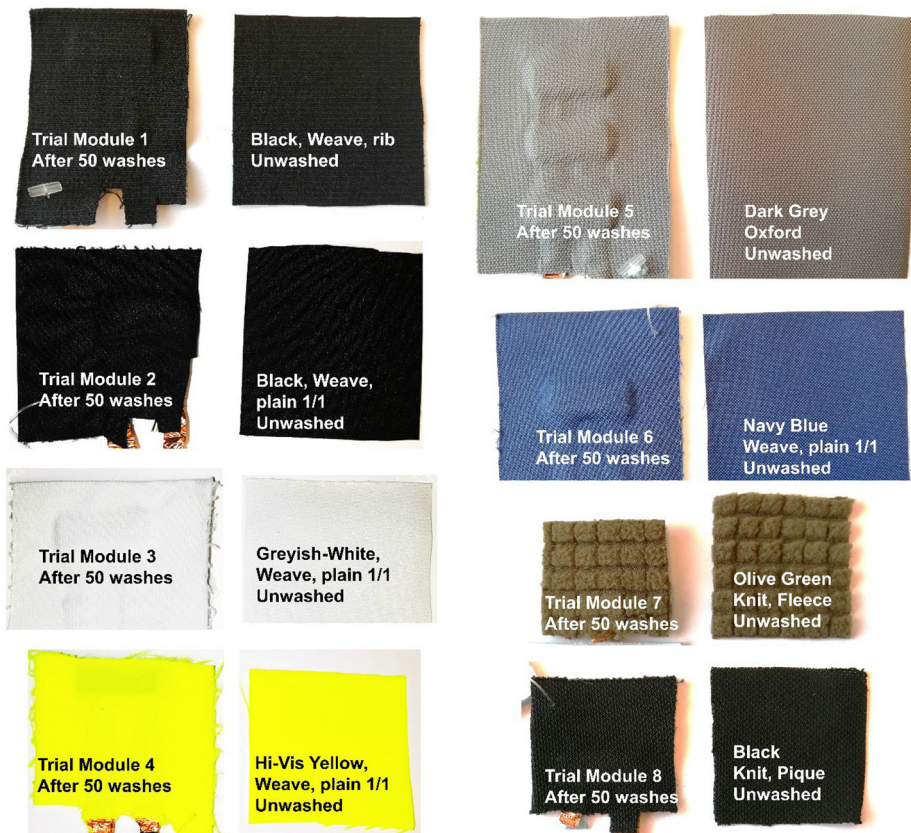
Figure 4. Textile solar modules before (right) and after 50 cycles of washing (left)
