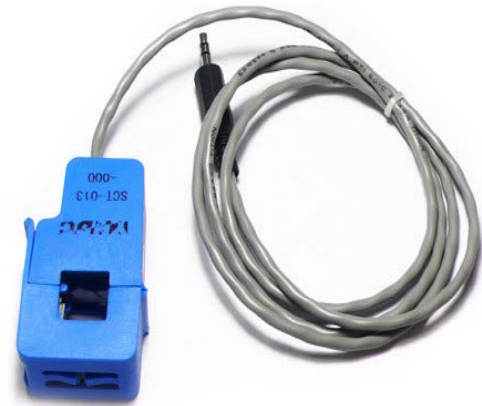
FIGURE 3. Split-core current transformer.
