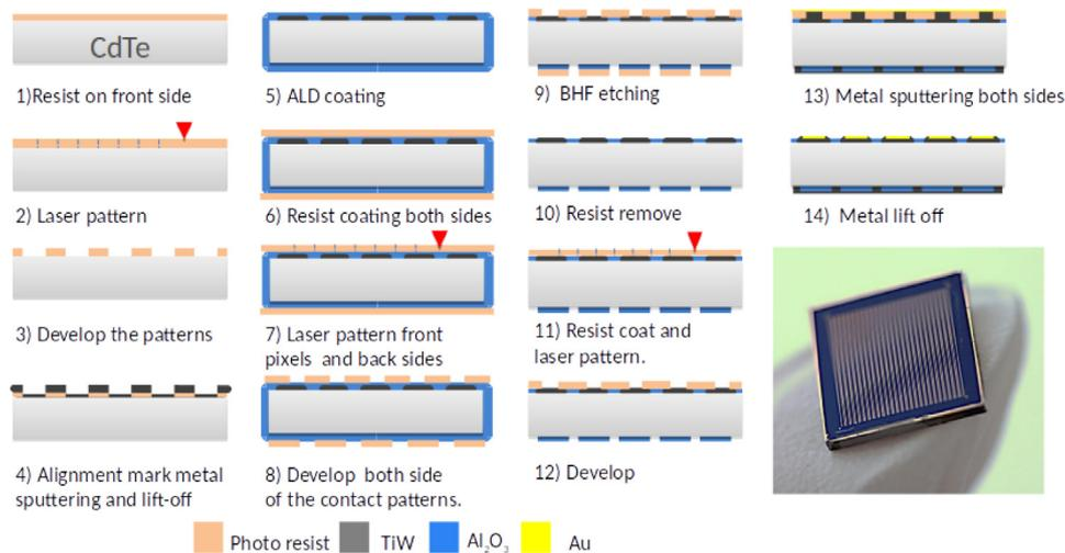
Fig. 2. Schematic of the processing steps (cf. [9]).
