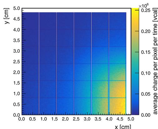
Fig. 6. Profile scan of a corner of the beam with a silicon pixel detector.
