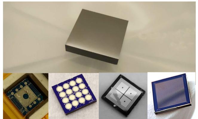
Fig. 4. *up*: raw CdTe,  $1 \times 1 \text{ cm}^2$  surface. *down*: four different test pattern structures. Detector with central optical opening; 16-pad structure; 4-pad structure; pixel detector.
