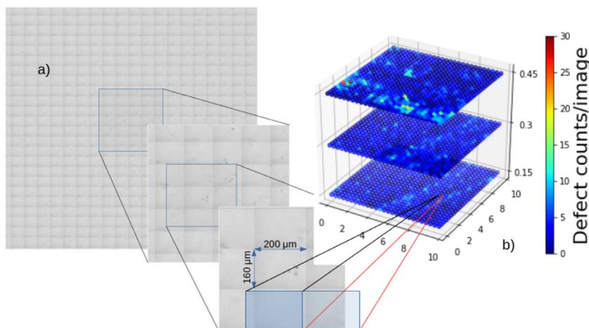
Fig. 1. (a) Stacked images of a raw CdTe crystal (b) visualization of defect counts/image for three crystal layers after NN evaluation, dimensions in mm.
