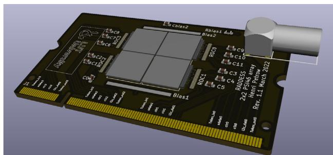
Fig. 7. Design of the PSI46 quad board, which will be able to host four pixel detectors tiled in a two by two array.
