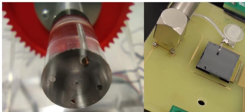
Fig. 5. A small rotating setup is used to obtain exemplary tomographic data (cf. [19]). *Left*: small phantom, connected to a gear wheel plus stepper motor for rotation. *right*: CdTe pixel detector connected to a read-out board.
