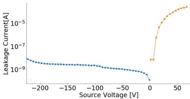
Fig. 3. Example IV curve for a CdTe pad detector. The amount of leakage current depends on the polarity of the bias voltage applied (cf. [19]).
