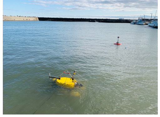
Fig. 3. Sea experiments at Hiratsuka Port, Japan. The yellow platform is the hovering AUV Tri-TON, and the red platform is the ASV BUTTORI.
