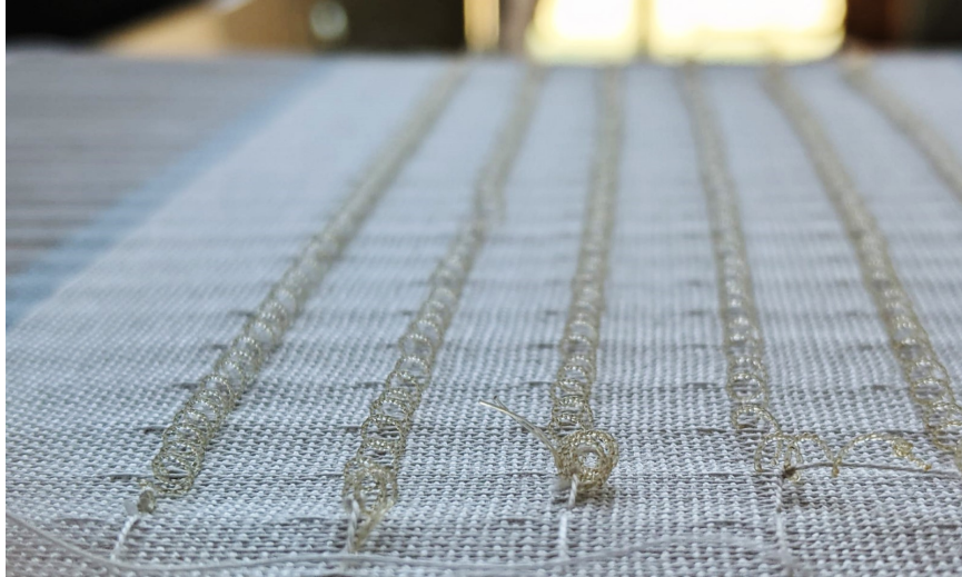
Figure 5. Fabric sample F6 on the loom. The fabric is woven with SZ, 2ply nylon coils and cotton yarns.
