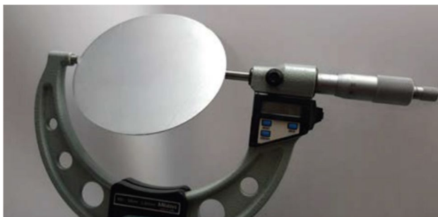
Fig. 17 Methodology for measurement of blanks
